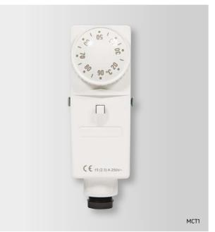
It is used for monitoring and controlling the temperature of the hot water stored within the hot water cylinder. When used with a thermostatic control for the heating circuit it will give boiler interlock providing a safety feature. It can also be used as a pipe thermostat in conjunction with a frost thermostat to ensure a boiler does not run uncontrolled during cold weather.
